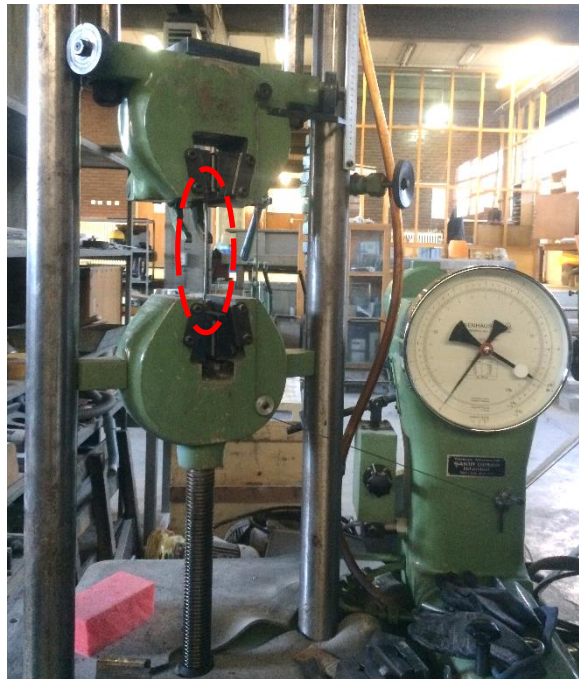
Figure 3.11. Tensile testing of conductor steel and aluminum wires
